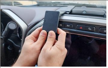
Installing the Rear Lip: Hook the thick angled edge on the back side of the mount onto the frame surrounding the center screen.
