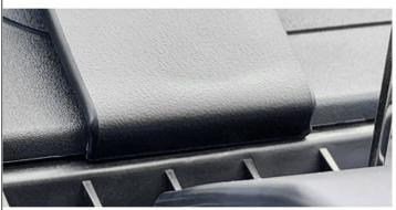
4. **Installing the Forward Lip:** Press the thin angled edge on the forward part of the mount into the seam between the top part of the dash and the inner part of the defroster vent.
